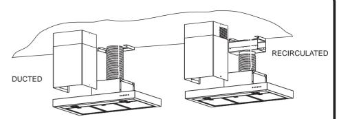
Before drilling any holes check the wall and ceiling are clear of any electrical cables, pipes etc. Fixing to a stud/noggin is recommended.
